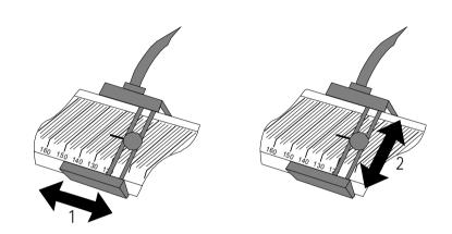
Now place the tip of the tab on the corresponding temperature line, e.g. on 135 °C for phenacetin (2).
